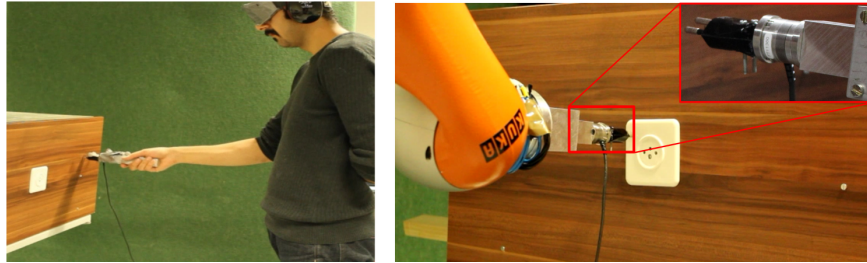
Figure 4.1: Peg-in-hole (PiH) search task. Left: A teacher is wearing ear defenders (to impede any hearing) and a blindfold. He first searches for the socket’s location and then attempts to establish a connection. Force and torque information is obtained from an ATI 6-axis force torque sensor at the end-effector of the tool held by the teacher. Right: The KUKA LWR4 robot equipped with the same force torque sensor and plug reproducing the teacher’s demonstrated behaviour.
